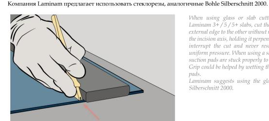
When using glass or slab cutters, normally preferred for *Laminam 3+/5/5+ slabs, cut the surface of the slab from one* external edge to the other without raising the tip of the tool from the incision axis, holding it perpendicular to the surface. Do not interrupt the cut and never resume cutting. Always apply uniform pressure. When using a slab cutter, make sure that the suction pads are stuck properly to the slab.
